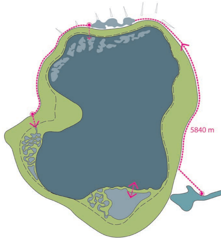
Preliminary design for water transfer via pipes along eastern and northern perimeter
